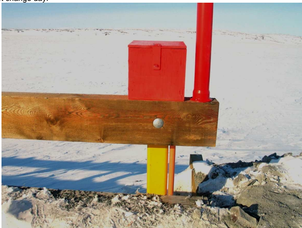
Photo 2: Thermister termination boxes. Bridge 2 north end. Note part of exposed cable is in a conduit.
